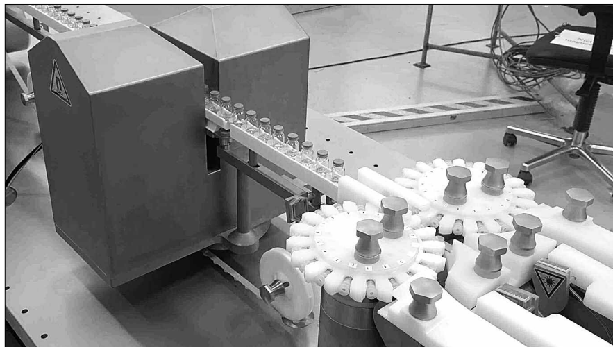
Vials passing through BOC Edwards' Non-Contact-Check-Weighing 7 (NCCW-7) system.
