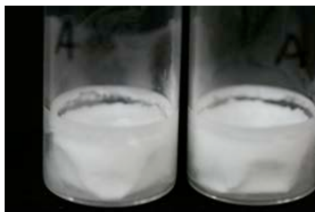
Figure 8. Appearance of a Sucrose / Tris Formulation When the Product Temperature Reached the Collapse Temperature of -37C During Primary Drying.
