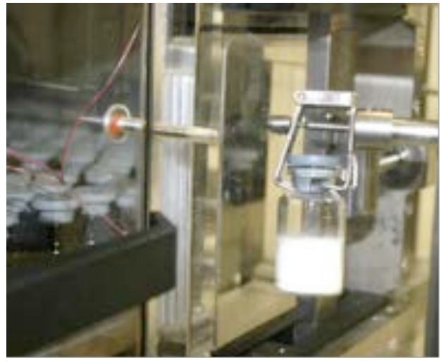
Figure 9. Collection of Samples from the Lyophilizer Using a Thief Sampler.
